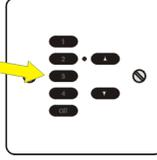
Press Off button to exit controller from programming mode
